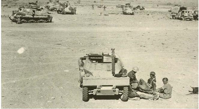
(Image courtesy of internet, source unknown) Description: Daimler Scout car in North Africa. Unfortunately no markings are visible so its not possible to establish the unit, note the Vickers gun used to increased sustained firepower
